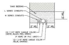
The conduit runs along and inside the SR-439 (USA Parkway) right-of-way from the intersection with US-50 to approximate engineer's station "USA" 696+35 for a total length of approximately thirteen (13) miles. The use of this conduit includes the proportionate use of the pull boxes installed with and integral to the conduit system.
